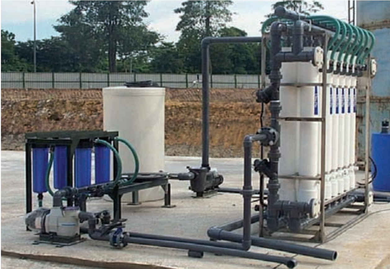
The water from Tiong Seng's first prototype portable water recycling system is used to wash vehicles, among others. 长成使用第一个原型污水再循环仪器把污水再循环, 然后用作洗车等用途。
